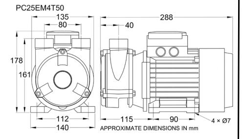
**Standard a.c. motor** 0.37Kw, 1380 rpm 400v/3/50Hz, totally enclosed fan ventilated IP55 enclosure. Contact your pump supplier for details of alternative motors
